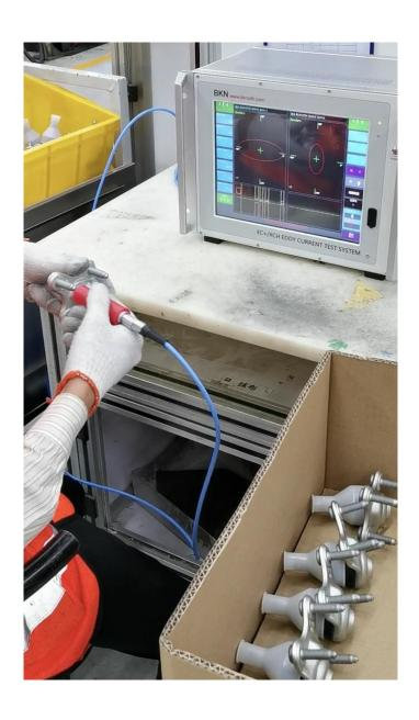
(1) Put two of the qualified workpieces into two contrast probes (A and B), keep the position consistent, press the center point of balance function, observe whether the red dot figure
