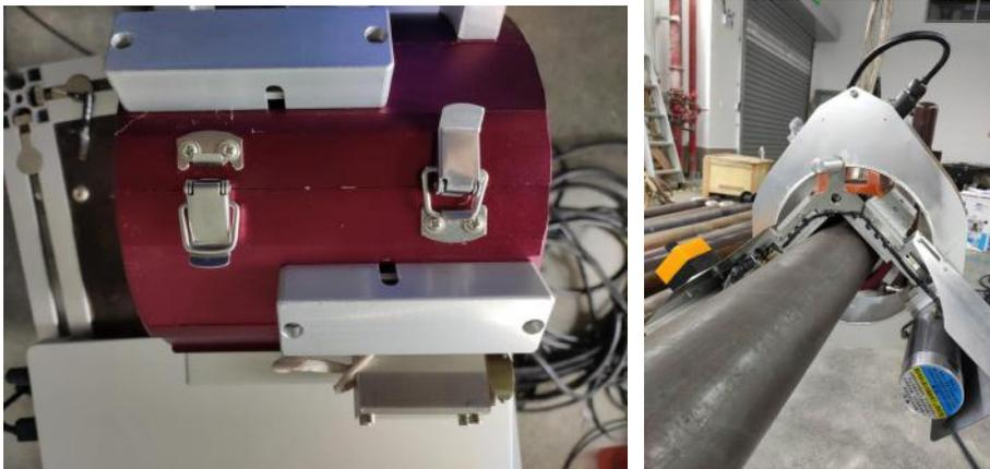
(3) Connect the probe 2, probe 3, probe 4, I/O interface, network communication, power supply line behind the instrument, and dial the power switch to the starting block. Note: Do not connect probe line in probe 1 position
