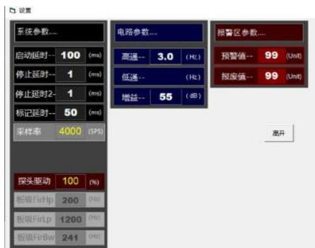
**启动延时-- 100 (ms)**: How long is the time delay after the motor switch is turned on to open the detection ms generally set to 50
