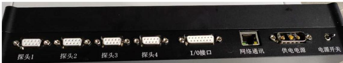
Then the other end of the probe line is connected to the probe socket, and the magnetic saturation power cord is connected to the magnetic saturation socket.
