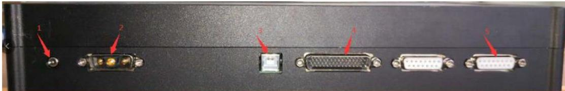
1. Turn the power switch to the left to turn on the power, and to the middle or right to turn off the power;
