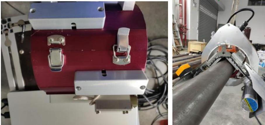
(3) Connect the probe 2, probe 3, probe 4, I/O interface, network communication, power supply line behind the instrument, and dial the power switch to the starting block. Note: Probe 1 position do not connect the probe line, probe 2,3,4 is a 6-channel detection system.
