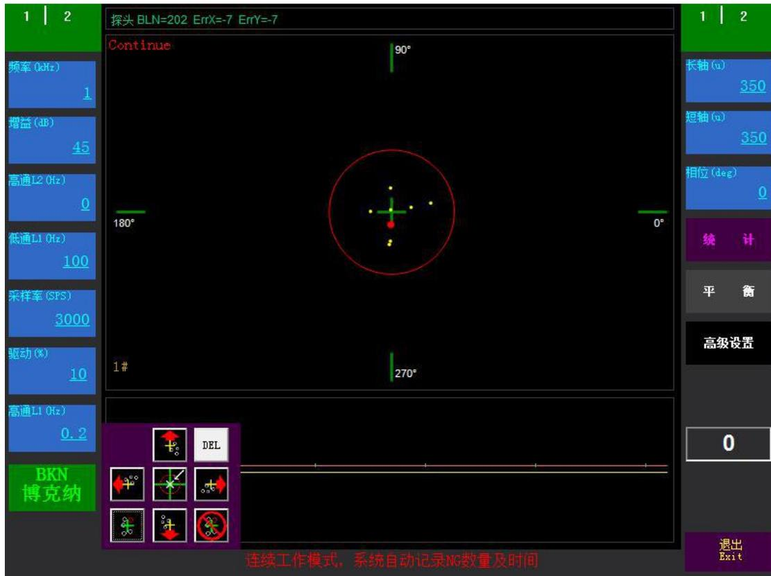
(3) At this time put unqualified workpiece, observe the distribution of red dot figure, adjust the alarm area range again (the figure of qualified workpiece is within the alarm range, the figure of unqualified workpiece is outside the alarm range, at the same time ensure that the difference between qualified and unqualified figure is large) as shown below.
